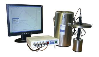
up. During cycle development, product temperature is often measured by inserting thermocouples or resistance thermometers into samples of product in the freeze-dryer, which provide an indication of what the product itself is experiencing during the process. This information can then be employed to refine processing conditions in the subsequent freeze-drying cycle, or indeed in the present cycle if the control system allows parameters to be changed 'on the fly'.
